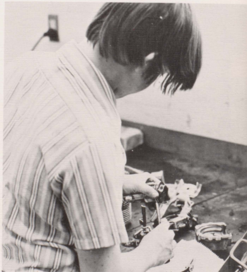
Taking the rings off the pistons in his motor is Dennis Dye.
