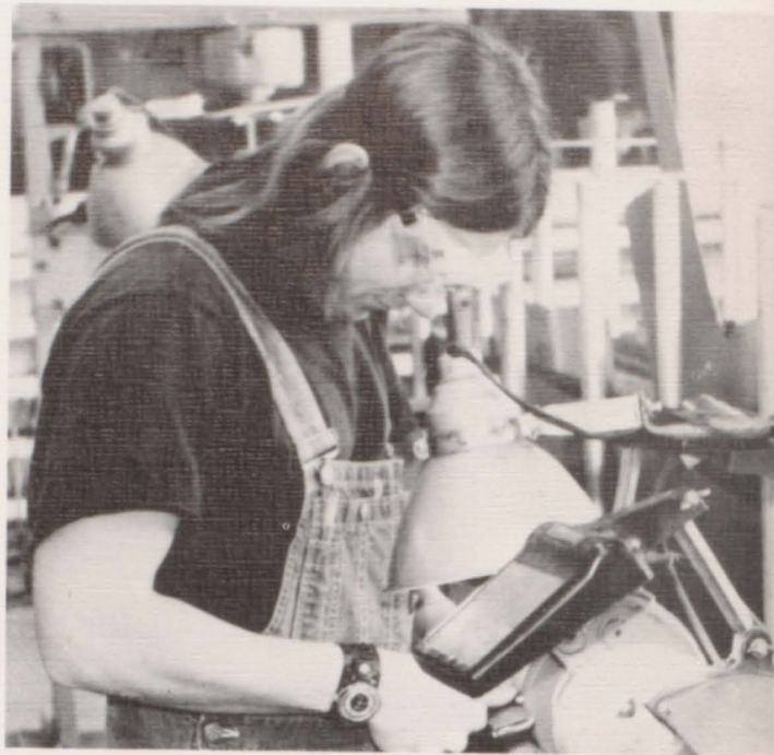
Industriously working at the emery wheel, or grinder, in metal shop, Paul Atkinson grinds a cutting tool for the lathe.
