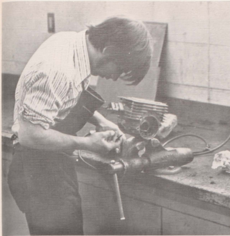
In small motor repair, Donnie White learns engine essentials he'll use now and in the future, as he removes the valves from his Honda.
