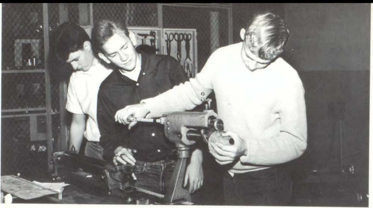
In Mr. Raymond Lesh's first hour Metals I class John Sellars is using the combination rotary machine to put
