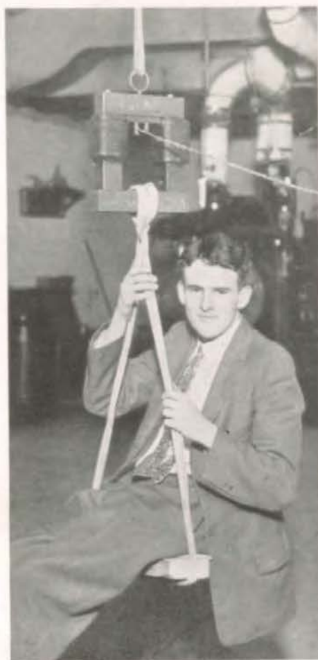
MAGNET MADE BY DONALD COLT. THE MAGNET WILL SUSTAIN A WEIGHT OF 350 POUNDS.
