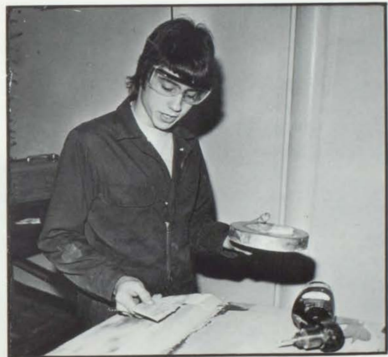
After welding a bottom patch panel onto a door, senior Billy Sterling uses plastic to straighten it out. (Photo by Kurt Branstetter)
