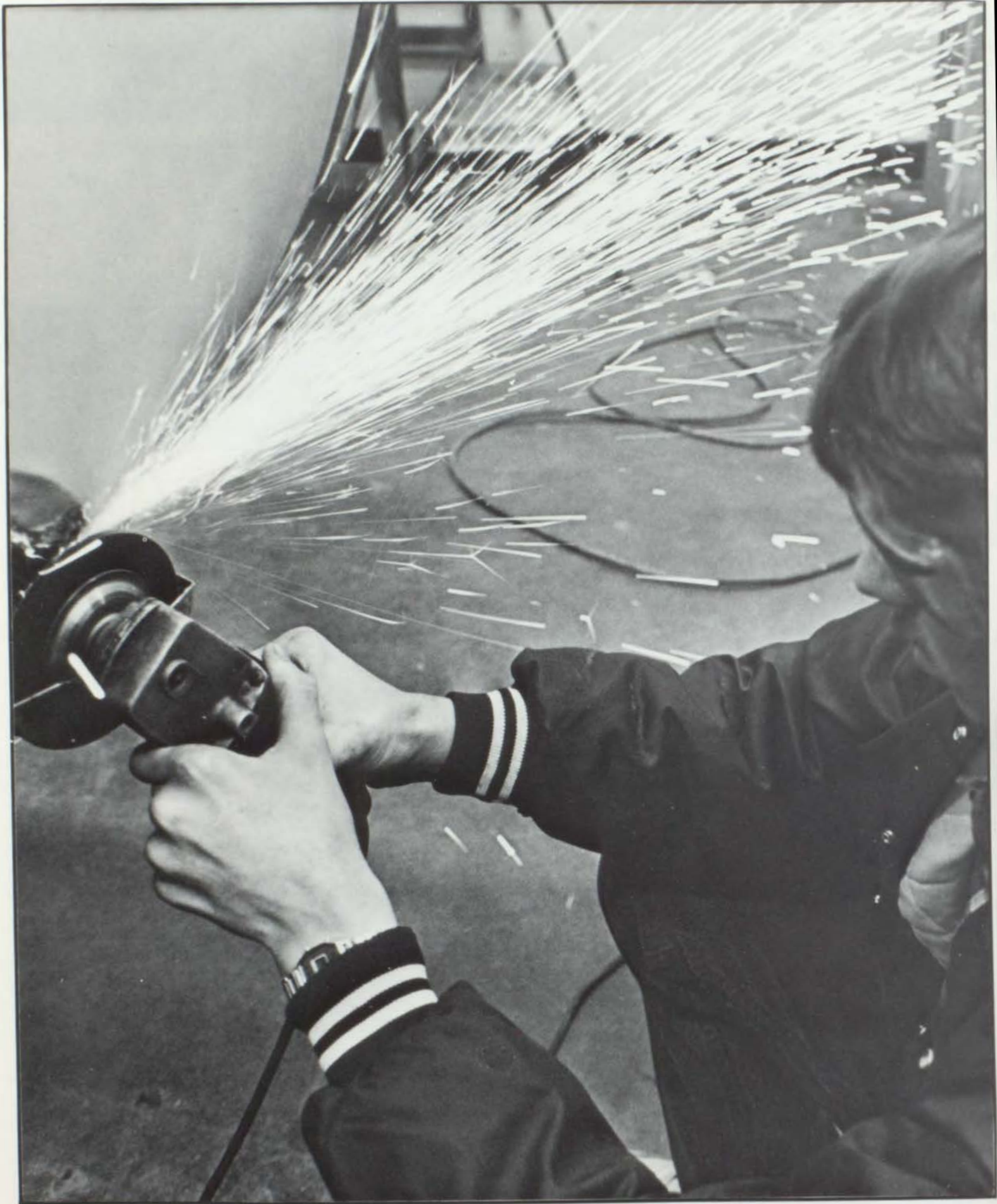
Fixing a mistake, senior Wayne Alderson grinds down a weld which was too big. (Photo by Kurt Branster)
