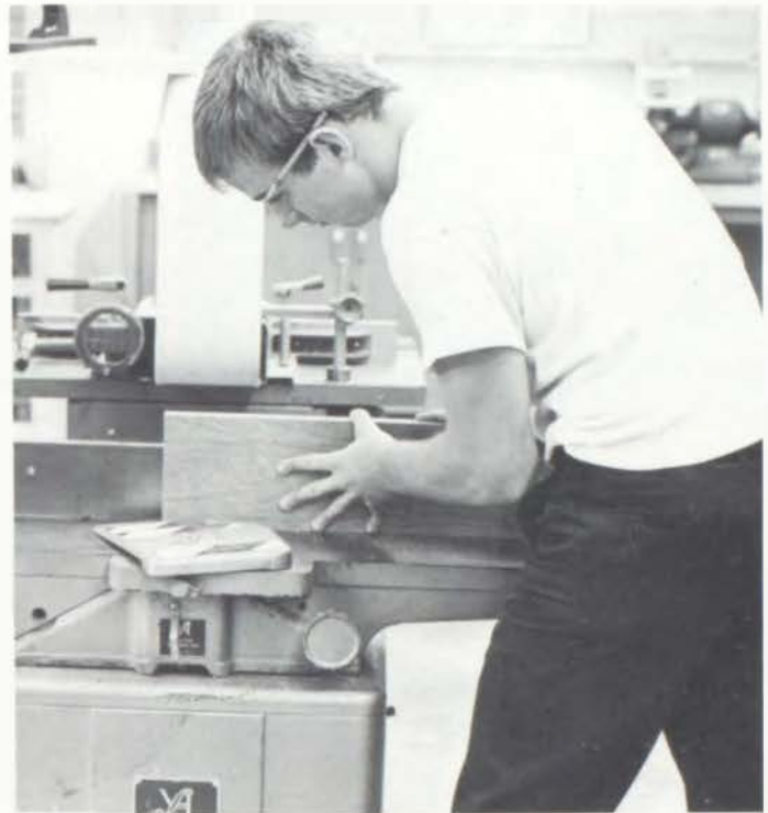
Senior John Moody uses the electric planer to square a block of wood in preparation for a project.
