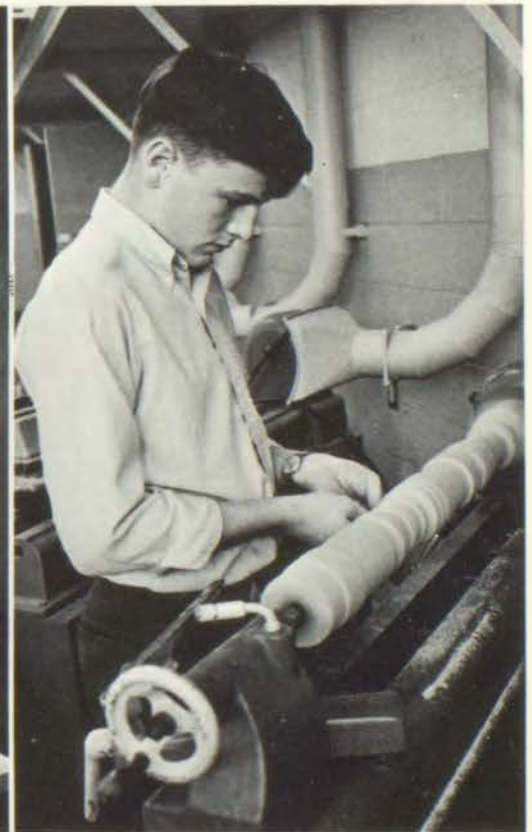
With the aid of a lathe, Mike Meaney sands his project to exact dimensions.
