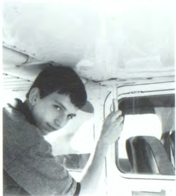
Brooks Kraft checks the fuel tank for any water that may cause some serious problems in flight.
