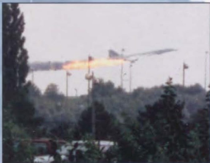
▲ In July, an Air France Concorde supersonic jet catches fire and crashes outside Paris, killing 113 people. The crash is blamed on metal debris which punctured the tires and damaged the fuel tanks.
