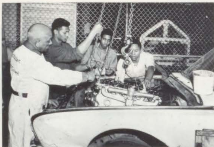
Removing a 1961 Ford engine to be overhauled. Mechanics Fredrick Lewis, Roosevelt Hargrove, and Simmie Crawford.
