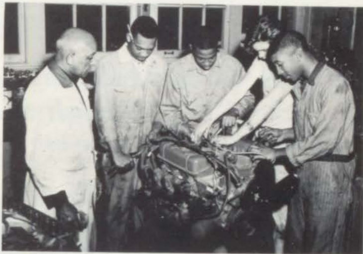
Removing cylinder head from a 1965 Buick. Eugene Moses, James Vivian, Chris Wheeler, and Rennie Gordon, Mr. J. K. Russell looks on.
