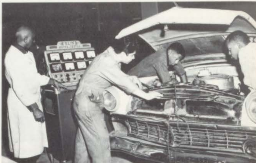
Mr. Russell observes the Removal of a generator for repair. Mechanics Darrell Jones, Clifton Lonymyer, Humberto Gallardo, J.K. Russell.
