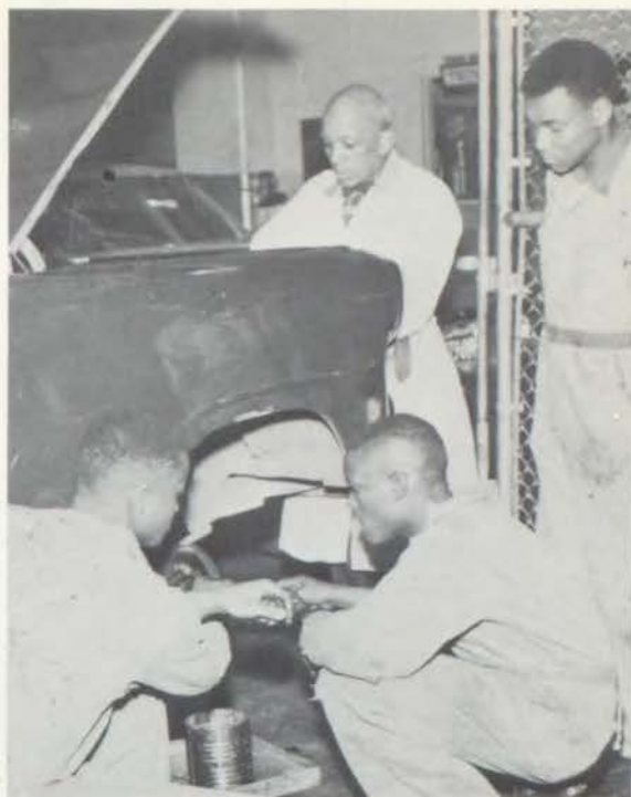
Installing brakes on a 1954 Ford. The mechanics are: James Poole, Jonathan McDonald, Francis Black, and Mr. Russell (instructor).
