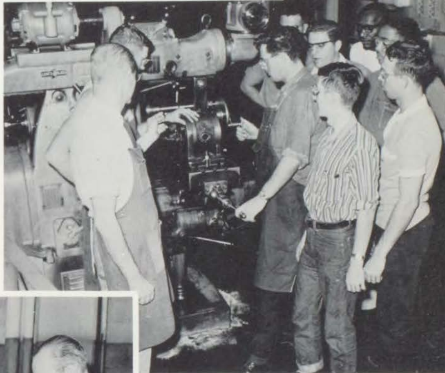
Gear cutting on the plain milling machine. Mr. Bridges, instructor, Gary Bacon, Edward Thompson, Milford McCónkendale, James Osterholt, Tony Elder, Rodney Athena and
