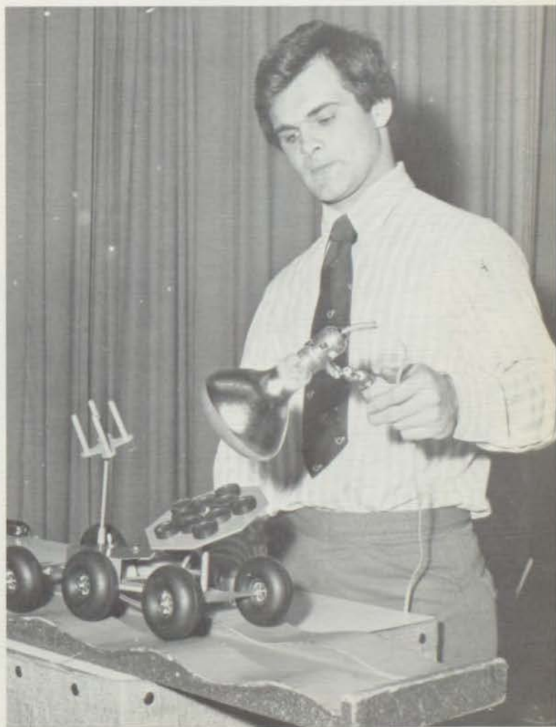
Light-rays are used to move vehicles with the help of special light cells on the top of this model moon car.
