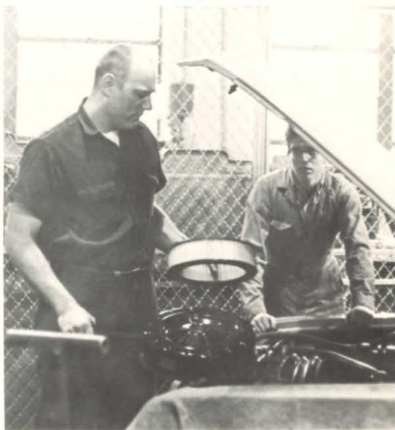
Eldon Flory, Mark Hunsinger, Stanley Flory and Ralph Kitsmiller utilize acquired skills to repair and replace parts of an engine taken from one of the vehicles that found its way to the experimental shop.
