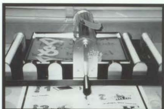
PTA purchased the "Accu-Cut" machine, used to make letters for signs and posters.
