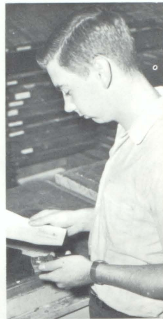
Pulling a proof really isn't as involved as it sounds. Mike Reams, who is just completing this job, explained that all you do is cover the lead set with ink and carefully place a clean sheet of paper over it. The next step is to roll a heavy object over it once and then lift the sheet of paper. If any mistakes were made in setting the type, they are easily found. Mike is now pulling the proof on the basketball schedule which he hand set.
